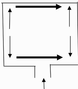
Feeding at the bottom forces larger currents through the bottom legs and creates horizontal polarization
