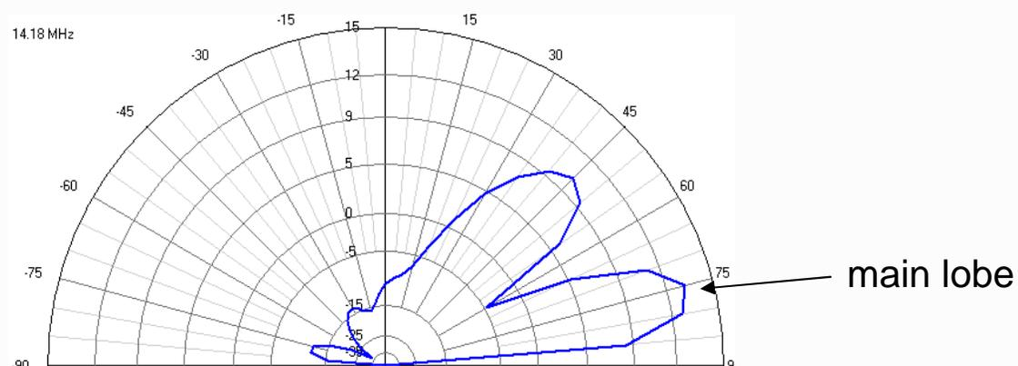
The “main lobe” of a directive antenna is the direction of the maximum radiated field strength from the antenna.
