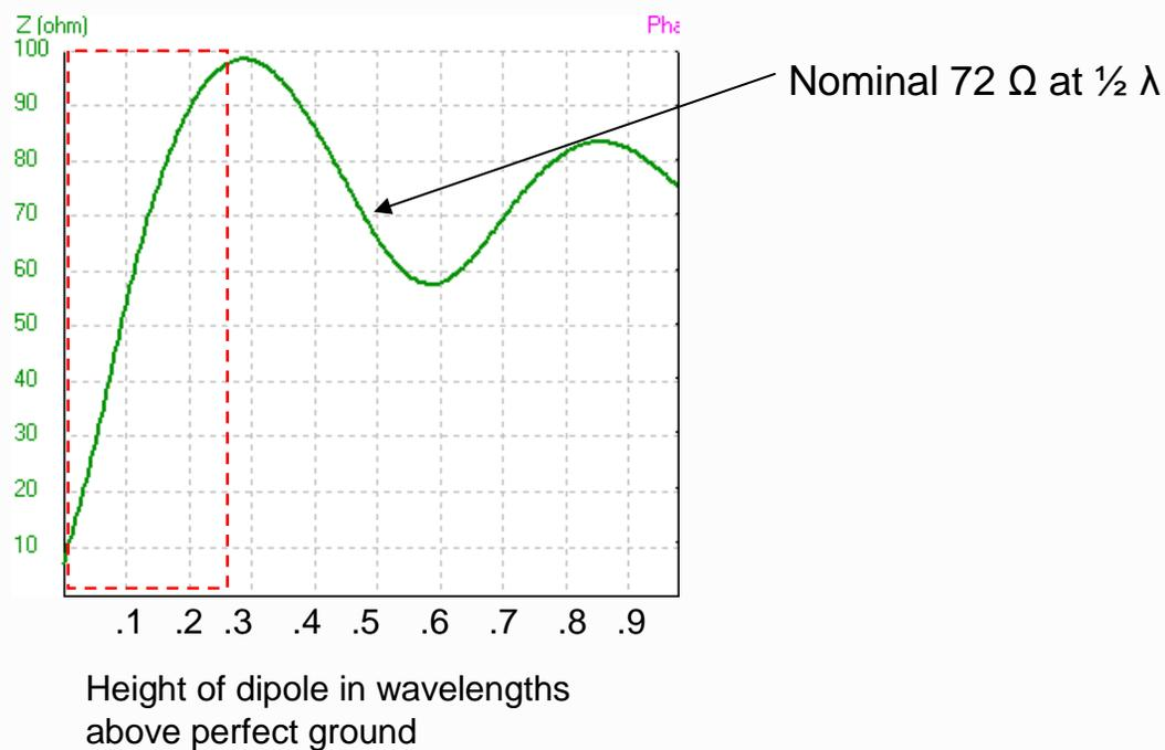
Height of a dipole affects the feed point impedance and radiation pattern. **As the height of antenna  $\downarrow$  below  $\frac{1}{4} \lambda$ ,  $Z_0 \downarrow$**
