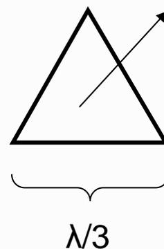
A loop antenna can be viewed as two dipoles. The radiation pattern for a full sized loop is broadside to the plane of the loop. If placed horizontally, most of the radiation goes straight up.
