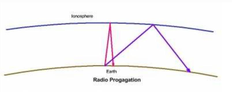
A dipole makes a very good NVIS antenna when it is close to the ground – **between 1/10 and ¼ wavelength above ground.**
