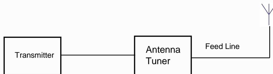
The Antenna tuner matches the antenna system impedance to the transmitter (or transceiver) output impedance. Antenna tuners are also called impedance matchers, transmatch, or antenna coupler.
