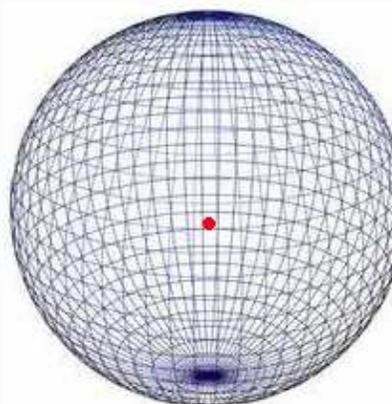
The Gain of an antenna describes the focusing of the antenna's radiated energy in the maximum direction and is measure dBi
