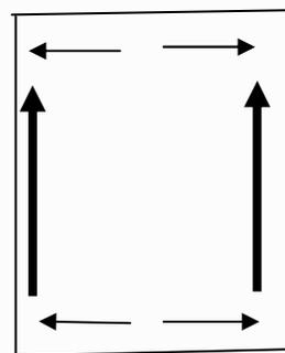
Feeding on the side forces larger current through the side legs and creates vertical polarization
