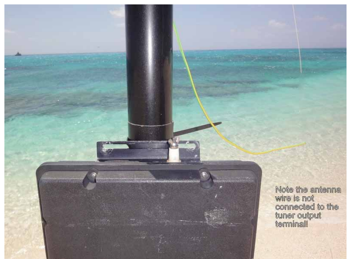
RTTY Station Antenna Coupler on the First Day We forgot to connect the antenna wire to the coupler's antenna terminal. We made about 100 QSO-s like that.
