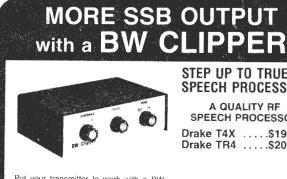
Put your transmitter to work with a BW Clipper. Installed in the IF strip, it increases average SSB output to a little below key down CW output. No non-reversible modifications.
