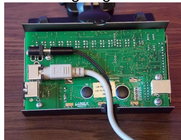
Showing Internal Connectors, Top or Bottom Cable Exit
